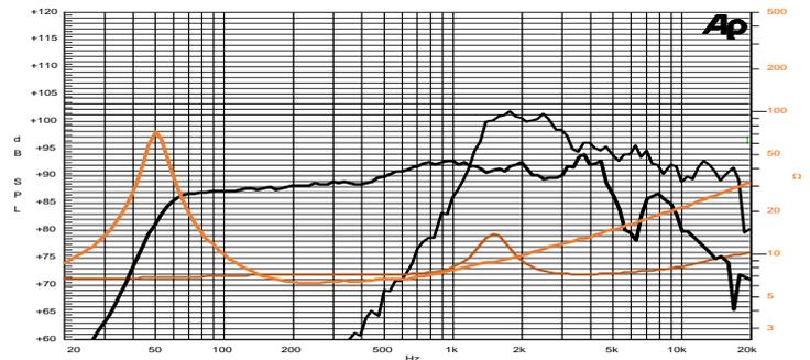
Frequency Response on 18 Lt @ 55 Hz Vented Box @ 1W, 1m
